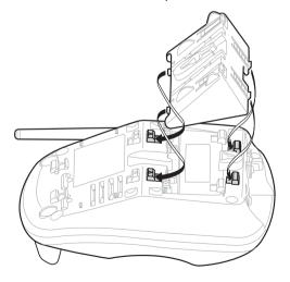
To put the phone on a slant, insert the clips into the middle clip slots. Then, tilt the bracket down so the tabs click into the upper tab slots.
